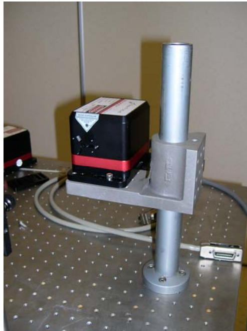
Figure 3.2. The New Focus Velocity diode laser operates through a range of 848nm to 854nm. It was mounted above the table to alleviate the need for multiple periscopes.
